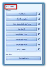
The Data Items pane allows you to create and modify data binding\* using drag-and-drop operations from the Data Query table alongside.
